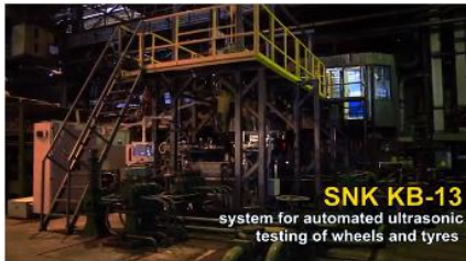
System of automated ultrasonic quality testing of wheels and rims SNK KB-13
