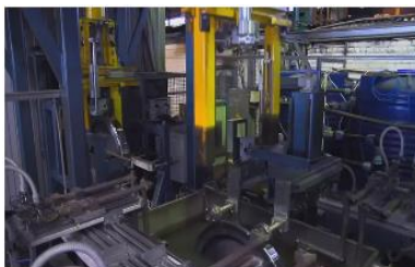
System of automated ultrasonic quality testing of wheels and rims SNK KB-13
