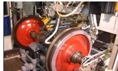
SNK KP-8 automated system for integrated nondestructive testing of railcar wheelsets
