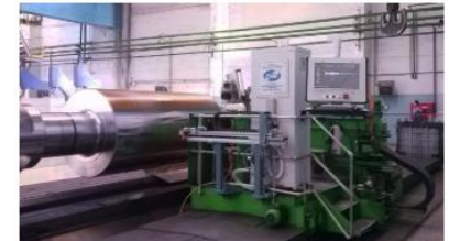
Automated ultrasonic and eddy-current system for mill rolls testing SNK B-35 (L)
