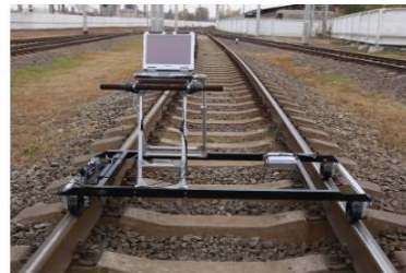
Eddy-current single-rail 8-channel flaw detector ETS2-77 for the track rails control
